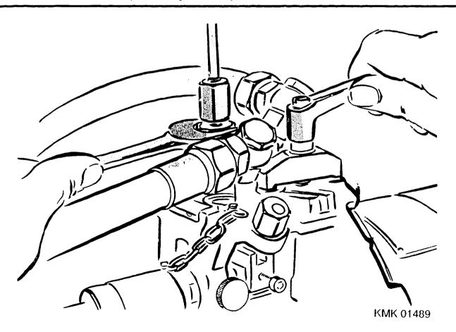
If the adjustment range within the fastening hole is not sufficient, perform correction at eccentric screw (arrow).
